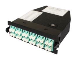
Hermesys pre-terminated fiber patch panel is dedicated to the Hermesys connector MPO/MTP conversion module installation card, the patch panel is divided into standard 19 "1U and 3U. in the 1U four conversion modules can be installed, with up to 96 cores, in the 3U 12 conversion modules can be installed with up to 288 cores.
