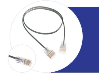
HydraX<sup>™</sup> 110 patch cords are used as jumper cords or end-user patch cords. These patch cords come in either 1 Pair, 2 Pairs or 4 Pairs and have 110 to 110 or 110 to RJ45 Plug. The standard lengths are 1, 2, 3 & 4 meters.
