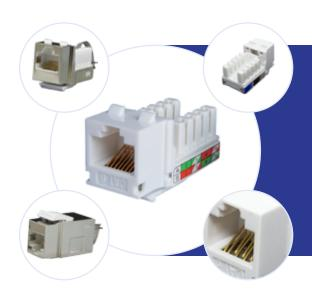
HydraX™ Cat. 5e dual IDC punch down modular jacks are designed for superior performance that meets or exceeds industry standard TIA/EIA 568A/B requirements. The modular jack will balance signal transmission of insertion loss and crosstalk from 1 to 250 MHz.
