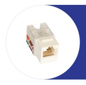
HydraX™ Cat. 5e 110 IDC punch down modular jacks are RJ45 8P 8C 50µm jacks suitable for 22-26AWG stranded and solid wire, compatible with 110 IDC punch down tools.
