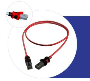
HydraX<sup>™</sup> Category 6A U/UTP patch cords are constructed of 24 AWG stranded conductor with an good performance modular plug on each end. Copper conductors in patch cable shall be twisted in pairs and separated by a special design separator to minimises the alien cross talk.
