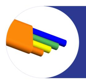
GryphonX™ flat bundle microducts are a part of an optical fibre cable blowing system which has been designed with expansion in mind and compatibility with existing technologies. The technique is based on laying the bundles of microducts first and afterwards blowing-in optical fibre cables.
